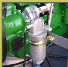
Oil change pump for routine oil change
