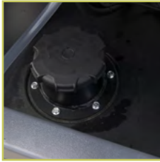
Tank filler wide tank refilling point
